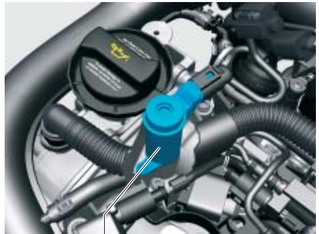
Inlet camshaft timing adjustment valve N205 S359_059
