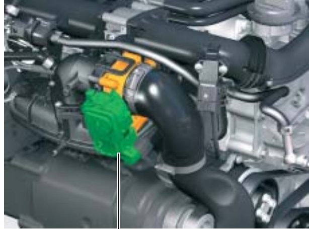
Throttle valve module J338 with angle sender for throttle valve drive G187 and G188
