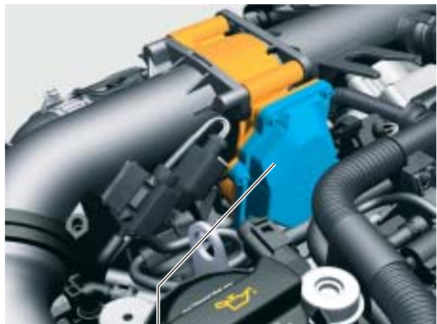
Regulating flap control unit J808 with regulating flap position control motor V380
