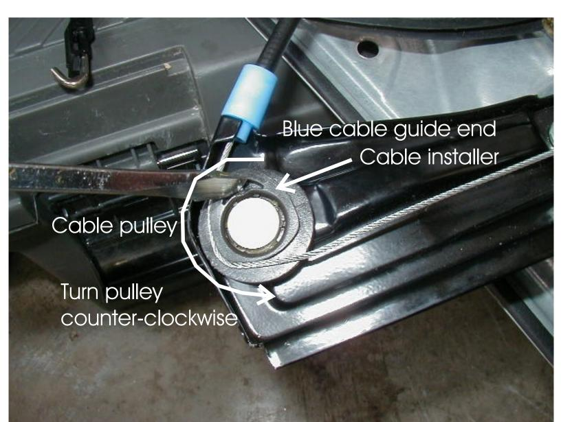
As you rotate the cable pulley, the cable will be placed into the cable pulley guide
